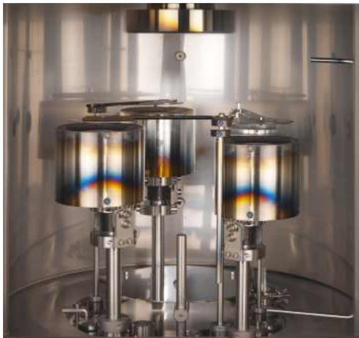
Sputter system with three height adjustable 75 mm magnetrons
