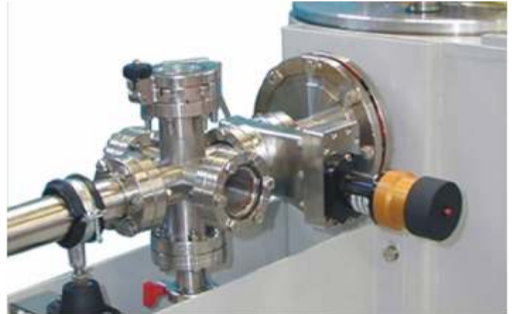
Coating chamber with load-lock assembly for two inch substrates
