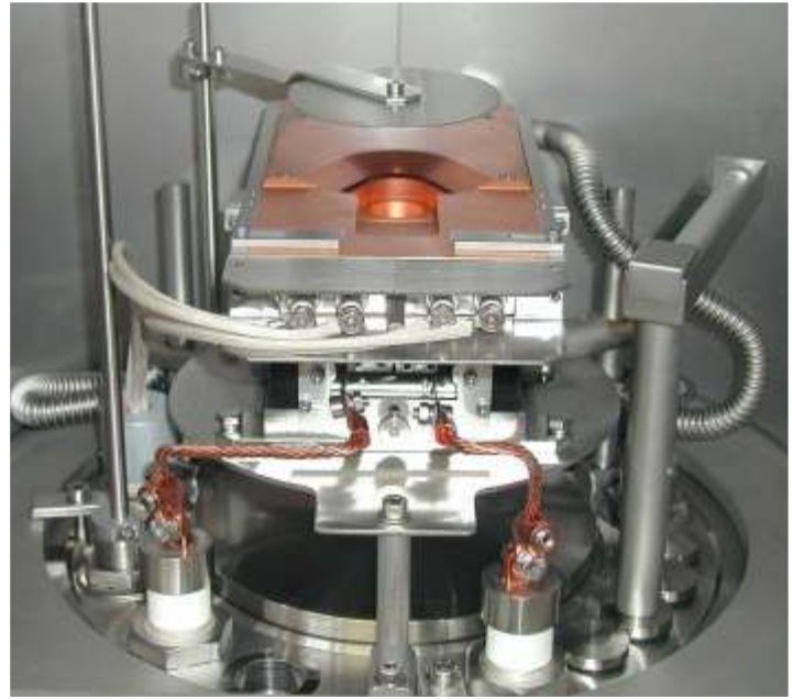
Interior of FL400 chamber showing EB3 electron beam source, two resistance sources and quartz lamp substrate heater.
